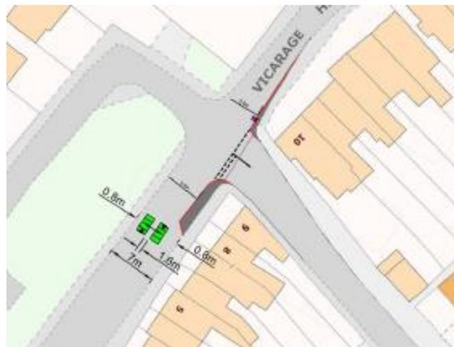
This moves the Give Way marking forward within the carriageway which increases visibility at this junction.
